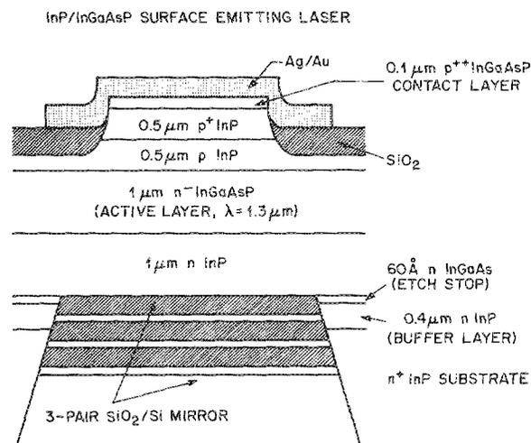
FIG. 1. Device structure of the InGaAsP/InP vertical-cavity surface-emitting laser.
