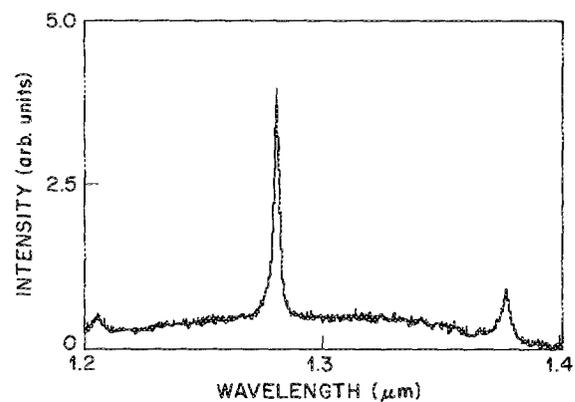
FIG. 5. Electroluminescence at room temperature measured from the VCSE laser. Three Fabry-Perot modes can be clearly seen.
