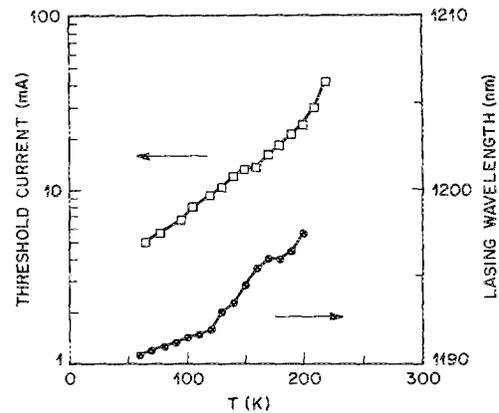
FIG. 4. Threshold current and the lasing wavelength as functions of temperature. The characteristic temperature  $T_0$  is found to be 87 K between 77 and 200 K.
