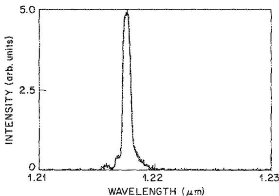
FIG. 3. Lasing spectrum of the VCSE laser pumped at  $I = 1.6I_{th}$  with 50% duty cycle at 77 K. The linewidth is 0.6 nm.
