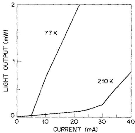
FIG. 2. Light output vs the current characteristics of the VCSE laser at 77 and 210 K. The pulse width and the repetition rate were 60 ns and 100 kHz, respectively.
